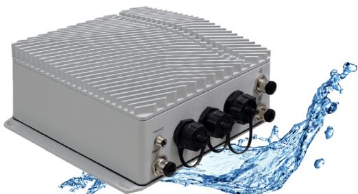
DFI's ECX700-AL Ruggedized Box PC is certified up to IP67 and supports industry-leading wide voltage and temperature to operate reliably outdoors. In addition, the system has waterproof connectors, further stopping any water from getting in. Due to the risks above to electronic circuitry from salt water, ECX700-AL's IP67 protection means that DFI's customers do not need to worry about electrical connections corroding or the overall system failing.
